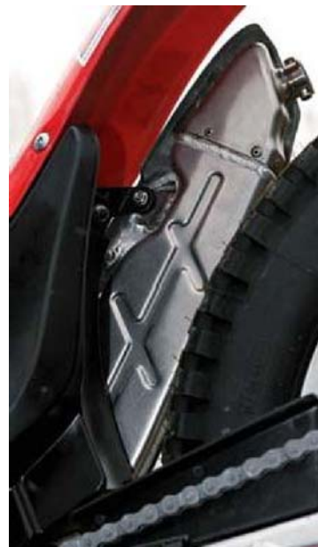
Montesa news 2007: the new silencer differs from the previous unit in that the exit has been modified to reduce the sound level. Plus, they have optimized the automatic decompression release along with the headlight and speedometer.
